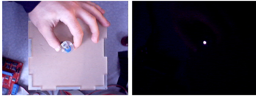
Figure 3.7: Overhead view of the Actuated Workbench from vision camera without IR filter (left) and with IR filter (right).
