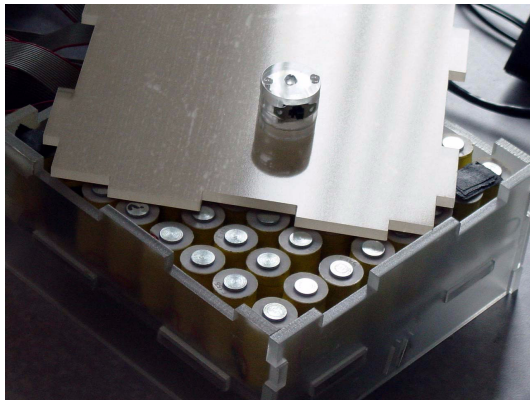
Figure 3.1: Our basic actuation platform contains a grid of 64 computer-controlled electromagnets.
